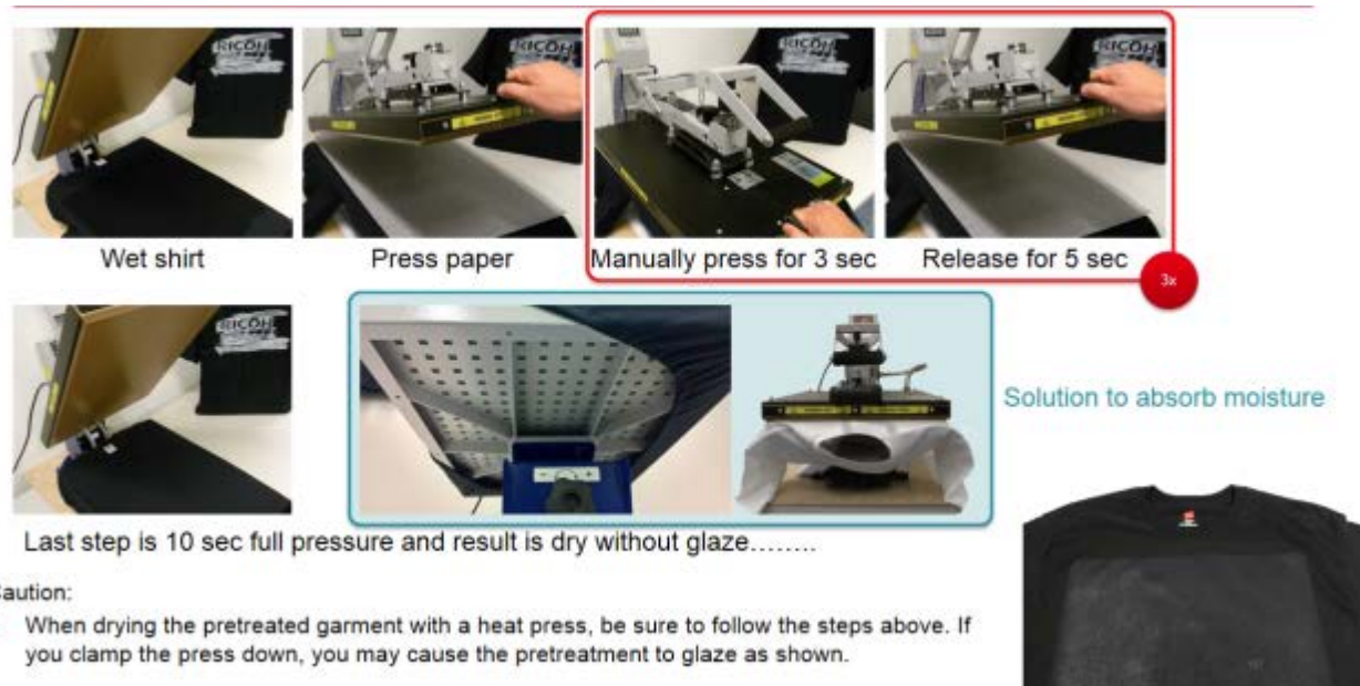
Figure 7.4-2: Heat Press Drying Procedure
